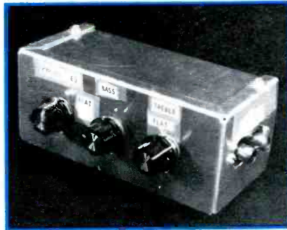
Figure 13. One example of a custom-built equalizer. It gave five degrees of bass boost, two treble decreases and three treble boosts. These passive circuits impart a loss of about 20dB.
