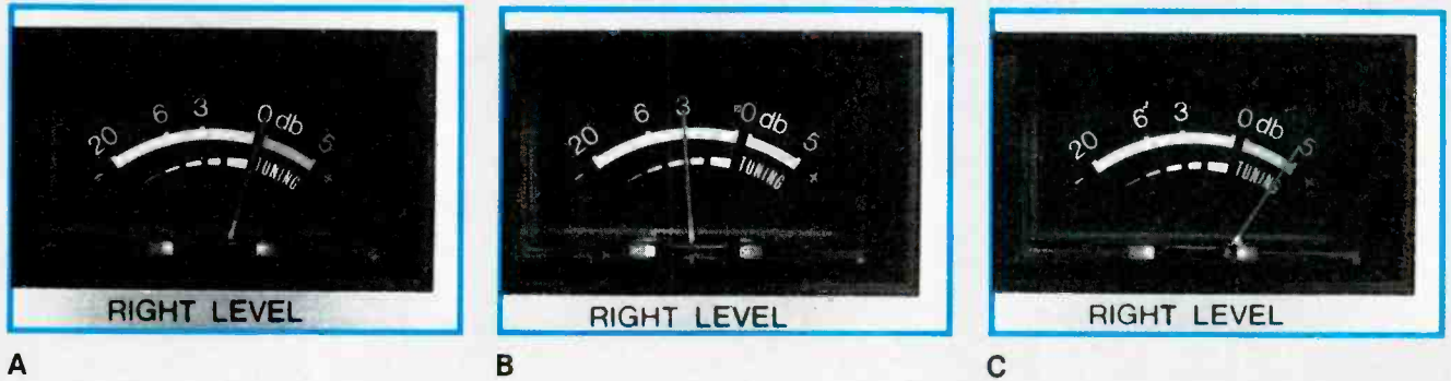
Figure 3. Recording levels displayed by analog meters frequently require offsetting when recording speech. (A) Zero level peaks usually are satisfactory with music. (B) When the pointer is vibrating rapidly around a lower reading, this might indicate correct gain for certain types of speech patterns. (C) Excessive levels normally should be avoided unless experiments show that this reading provides normal recording levels for certain kinds of human speech.
