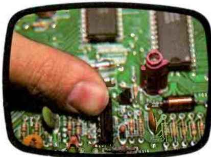
The body of the IC is bent back and forth until the pins on the other side snap off. This produces a clean break, and a new hex buffer can then be soldered right to the top of the motherboard.
