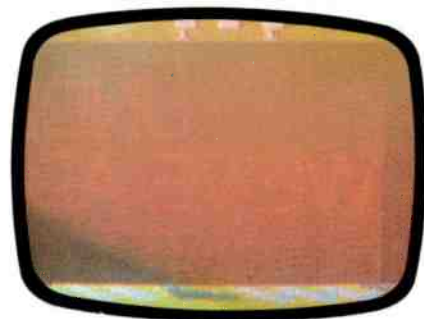
Smearing and distortion in this example was the result of a defective voltage regulator.
