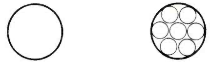
Figure 4. A solid conductor may be replaced by a stranded conductor of the same gauge size. If the conductor at the left is 22Ga, the stranded one at the right might be listed as 7x30Ga.
